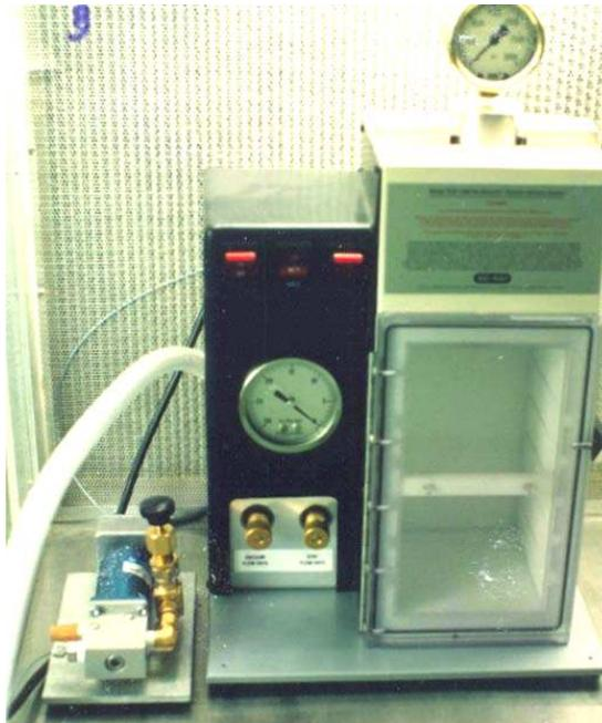
Fig 1: Micro projectile bombardment facility (BIORAD)
